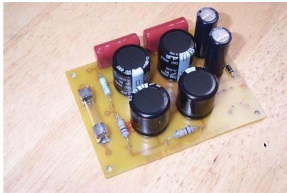
PAS Power Supply Capacitor Board
